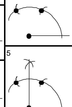
construct a perpendicular from C
